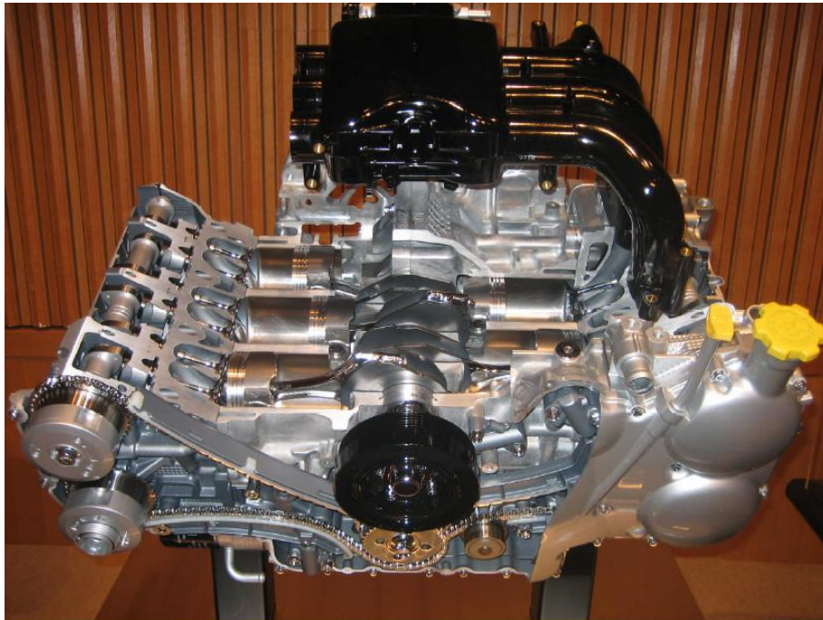
Subaru Boxer Engine, 6 cylinder, 3.6l; 256 hp@ 6000rev/min; 247 lb-ft @4800rev/min
