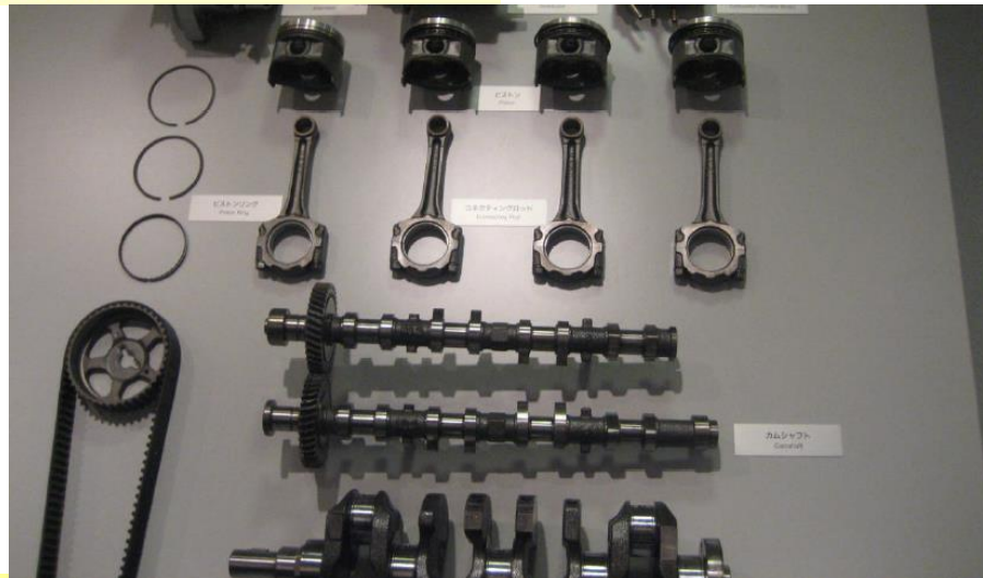
Pistons, connecting rods, camshafts, crankshaft, camshaft belt drive off crankshaft
